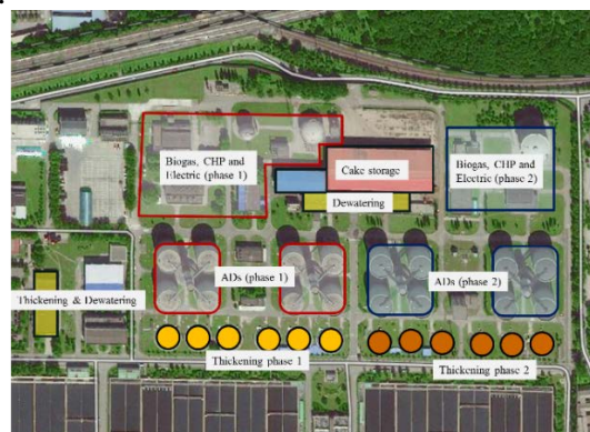
Fig. 2. Gaobeidian – original sludge treatment facilities (with 16 digesters until 2016)
